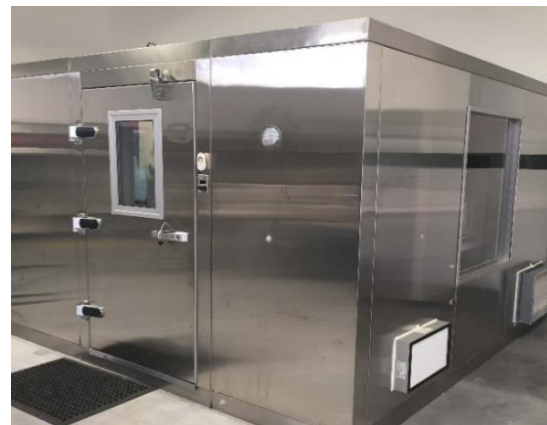
Figure 5. Stainless steel secondary aerosol containment chamber, which housed the 300-liter primary aerosol test chamber.
