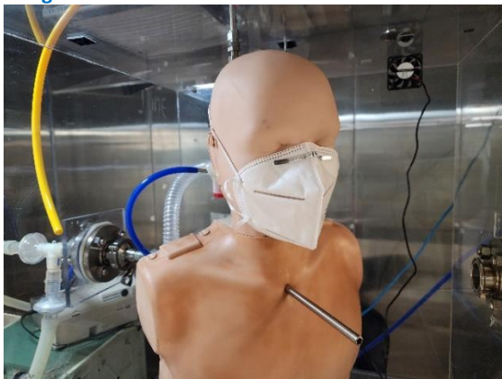
Figure 4. Image of the AccuMed NIOSH certified N95 Mask on The Ventilated Mannequin.
