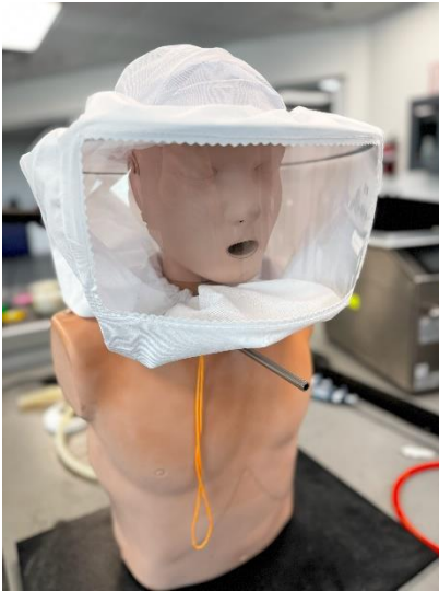
Figure 3. Image of the MyAirHat on The Ventilated Mannequin.
